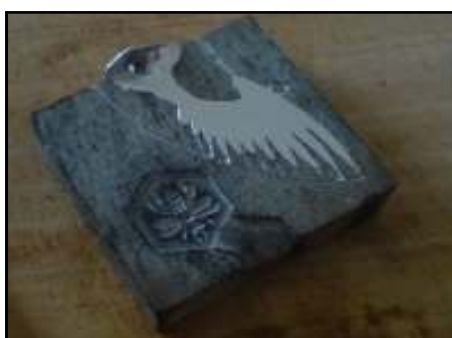
Mould after pour, with back removed.
